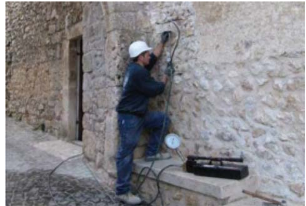
Figure 6. Example of double flat jack test.
