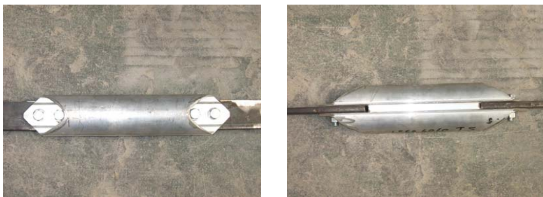
Figure 2. Photos of the EN AW-6060 T6 extruded prototype
