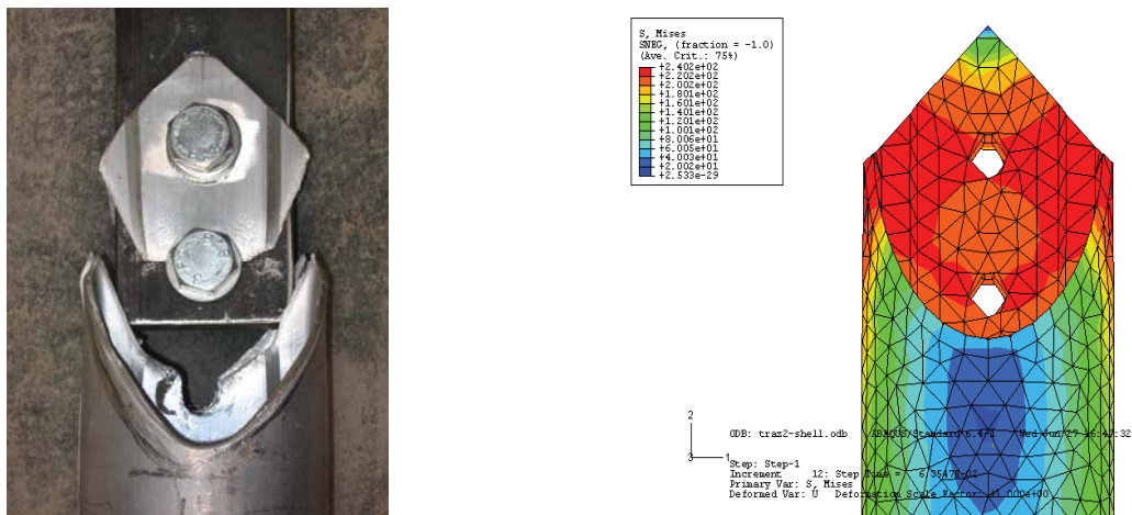
Figure 4. Experimental-numerical comparison in terms of final failure mode
