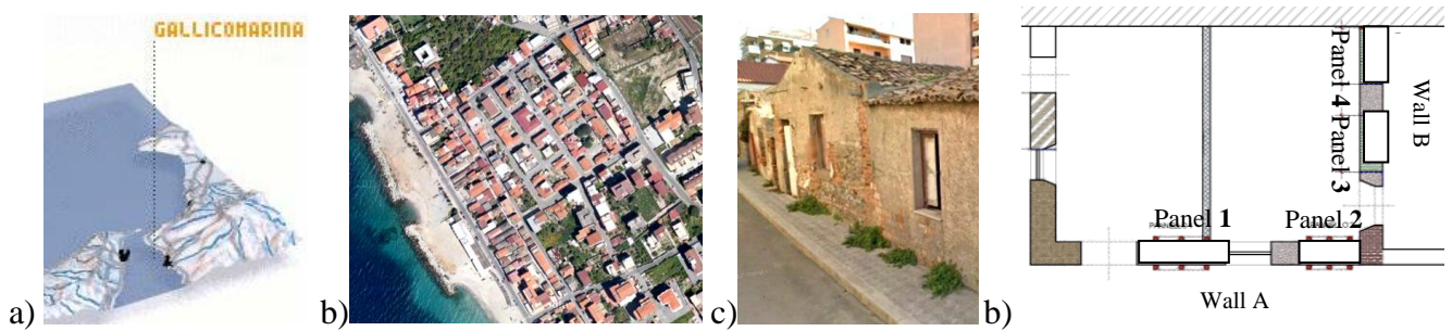
Figure 7: Experiments in Gallico Marina (Rc) Italy: a) the geographical placement; b) the ancient city of Gallico Marina; c) the case study; d) The building plane: (Wall A) the unreinforced panels [1 and 2] and (Wall B) the reinforced ones [3 and 4].
