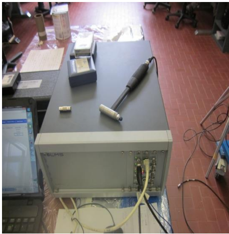
Fig. 5 Dynamic contact test instrumentation
