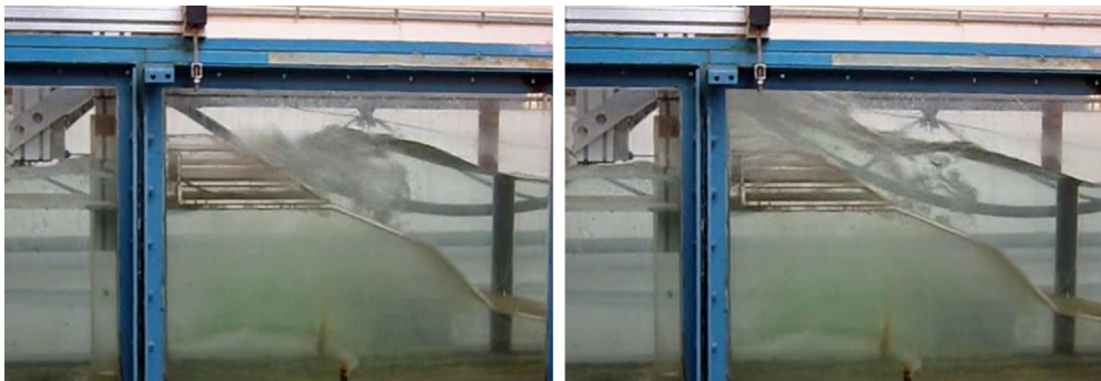
Fig. 13. Surging breaker with large wave height ( H=0.16 m, T=2 s). Left panel: the crest of the wave reaches the dissipation area at the toe of the front. Right panel: the water tongue hits the SSG and overtops the roof.
