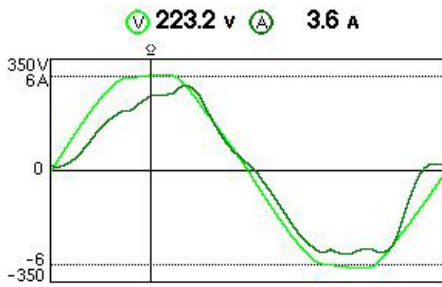
Fig.37 Air-condition device's voltage and current (heating mode).
