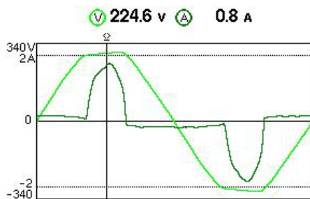
Fig.21 PC and monitor's voltage and current (hard disk drive access).
