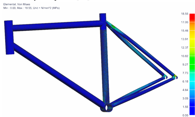
Fig. 11. Results of the FEM Analysis (Stress) on the A-Frame.
