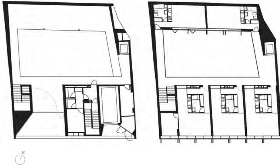
3. Project plans: ground floor, with courtyard opening, and 5th floor, with the units on the perimeter and courtyard in the center.
