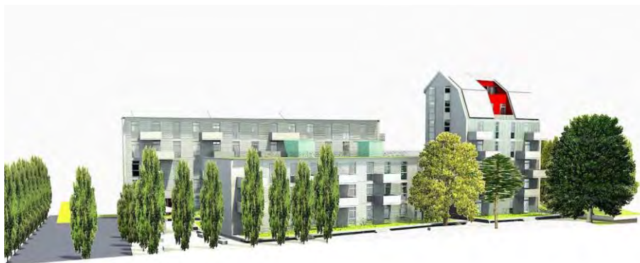
4: 1+1>2: view from south. The full-grown existing trees are on the right. The different height of the volumes allows sunlight into the courtyard while optimizing building costs.
