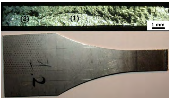
Fig. 15. Fracture surface of the joint welded at 17 mm/s and 0.8 kW (cycles to failure = 6985, % of UTS = 80%). Propagation surfaces of the main (1) and secondary (2) crack are evidenced.
