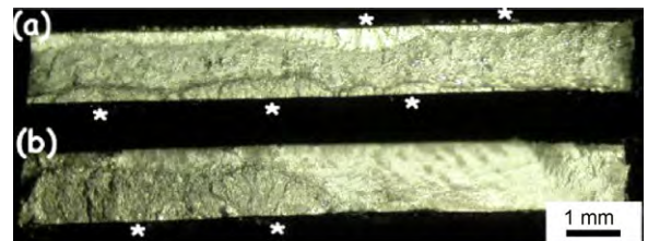
Fig. 16. fracture surfaces of the joint welded at 25 mm/s and 1.2 kW. (a) cycles to failure = 610, % of UTS = 80%, (b) cycles to failure = 29,890, % of UTS = 40%. Asterisks indicate the crack initiation points.
