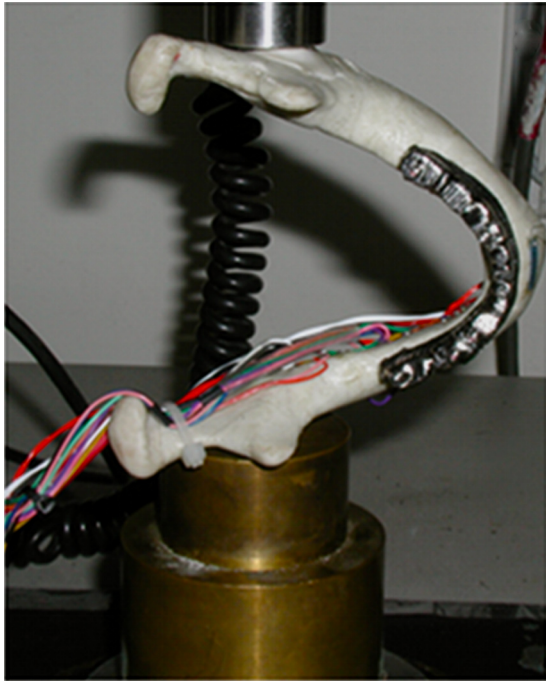
Fig. 2. Experimental set-up for the in vitro testing of mandible.
