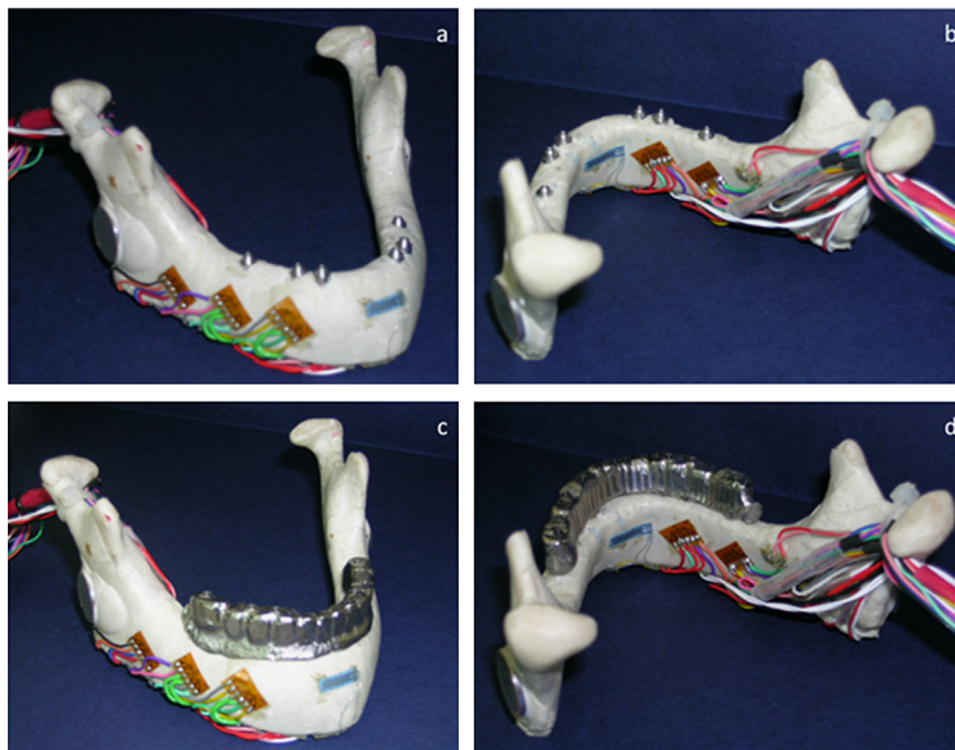
Fig. 1. Anisotropic mandible model instrumented with strain gauges and rosettes: a) vestibular perspective showing implants positioning into the mandible, b) lingual perspective, c) vestibular perspective showing the mandible rehabilitated with titanium full arch bridge, and d) lingual perspective showing inner strain gauge and rosettes.
