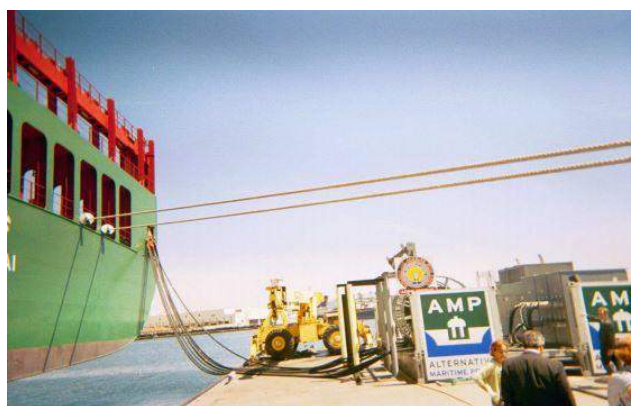
Fig. 4 Cold ironing arrangement in a Chinese port
