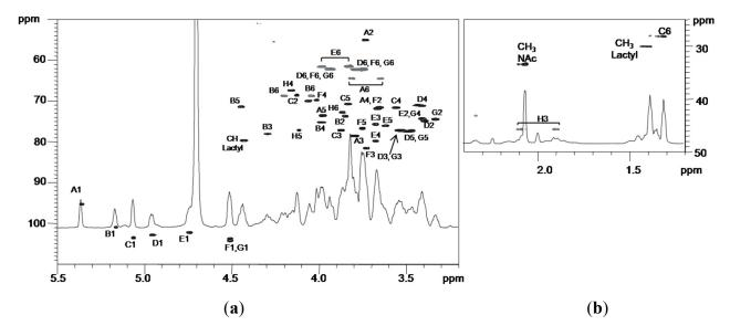
**Figure 5.** Anomeric/carbinolic (a) and aliphatic regions (b) of  ${}^{1}\text{H}-{}^{13}\text{C}$  DEPT-HSQC spectrum of OS core of the LOS from *P. arcticus* strain 273-4. The spectrum was recorded in D<sub>2</sub>O at 310 K at 600 MHz.
