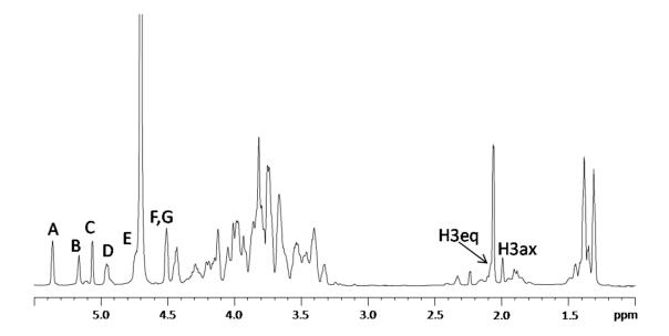
**Figure 4.** <sup>1</sup>H NMR spectrum of the core oligosaccharide (OS) obtained by mild hydrolysis of LOS. The spectrum was recorded in D<sub>2</sub>O at 310 K at 600 MHz. The letters refer to the residues as described in Table 2 and Scheme 1.
