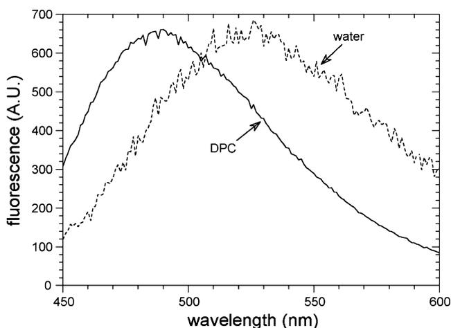
**Fig. 1** Fluorescence spectra of 1,8-ANS. The spectrum in water has been amplified 60-fold as compared to the actual one
