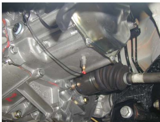
Fig. 4. Acceleration measure point
