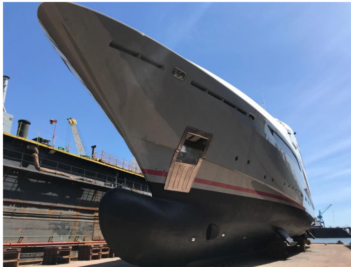
Figure 4. Conventional bow with bulb example.
