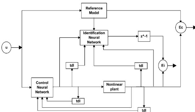
Fig. 6. Indirect adaptive control using neural networks.
