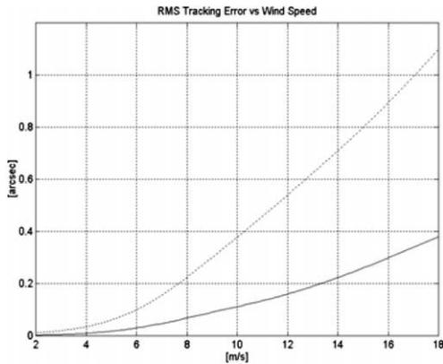
Fig. 13. Control model RMS tracking error vs. wind speed ( $\alpha = 0.63$  case) (VSPI upper line, NVSPI lower line).
