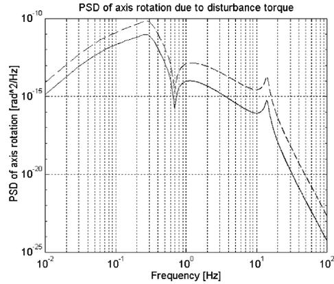
Fig. 11. PSD of axis rotation due to the wind disturbance torque  $S_\theta(f) \times (\alpha = 0.98$  dashed line,  $\alpha = 0.63$  continuous line).
