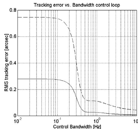
Fig. 12. Tracking error vs. bandwidth of the control loop ( $\alpha = 0.98$  dashed line,  $\alpha = 0.63$  continuous line).
