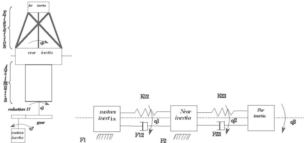
Fig. 9. Telescope model (main axes) block diagrams.
