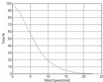
Fig. 10. Time% vs. wind speed in Paranal.
