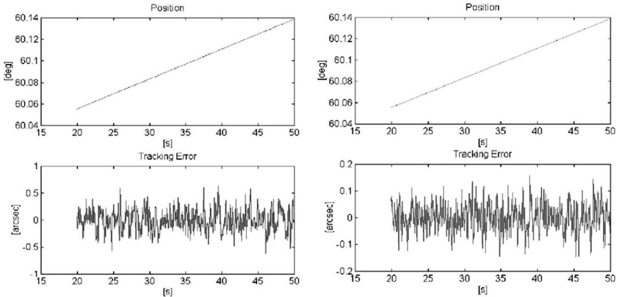
Fig. 15. Altitude axis test. Tracking RMS result using VSPI (left figure) and NVSPI (right figure).
