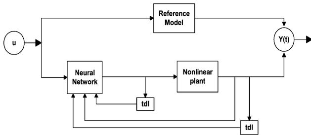
Fig. 5. Direct adaptive control using neural networks.
