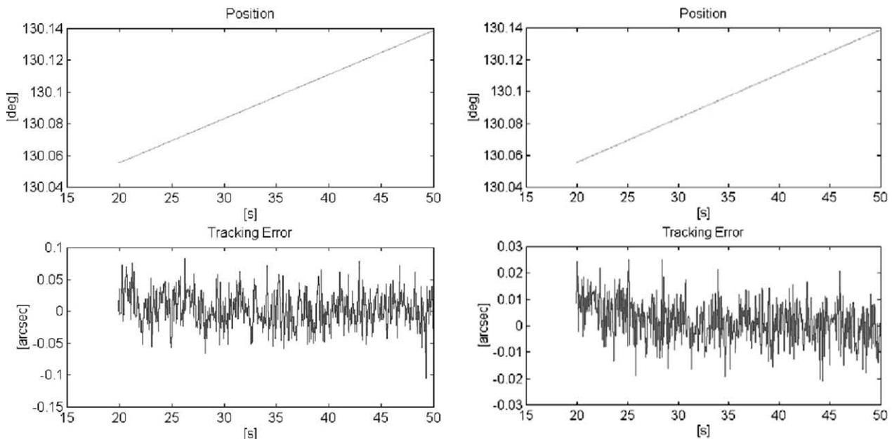
Fig. 14. Azimuth axis test. Tracking RMS result using VSPI (left figure) and NVSPI (right figure).
