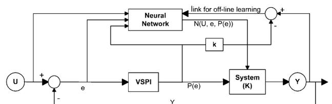
Fig. 7. NVSPI off-line learning control scheme.
