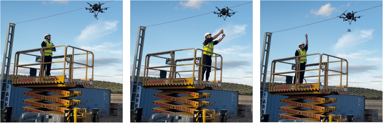
Figure 13: Tool delivery demonstration. Left) the gesture "palms together" causes the pulley to descend. Center) the operator retrieves the tool. Right) the gesture "arm up" commands the pulley to rise.
