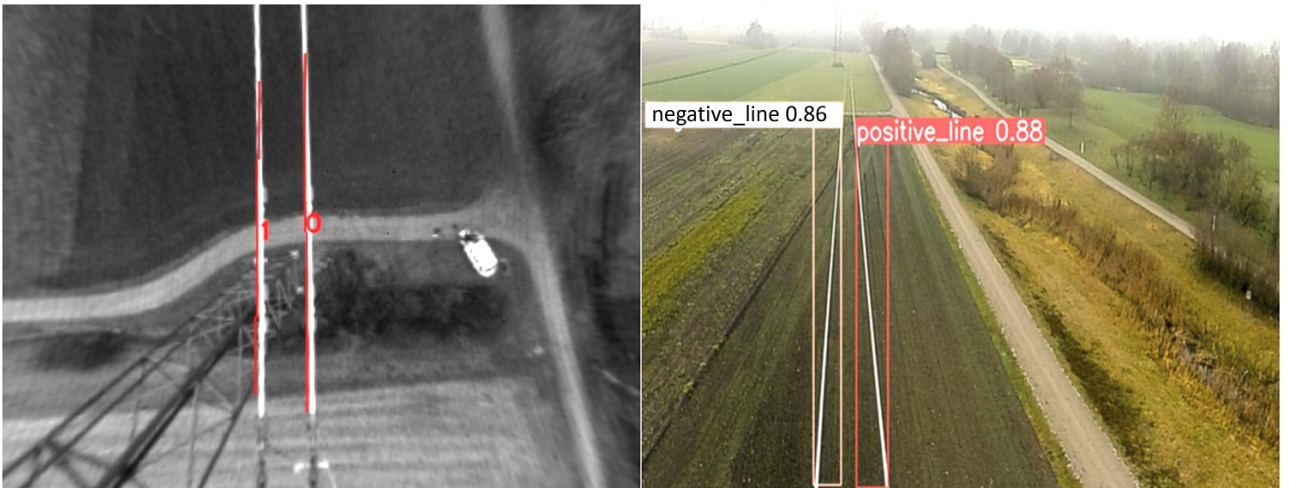
Figure 6: Left) output of the event-based tracker [33]. The algorithm assigns to each tracked line a unique ID. Right) output of the RGB-based tracker [12]. The algorithm assigns to each tracked line its inclination (positive or negative), a confidence score, and a unique ID (not visualized).
