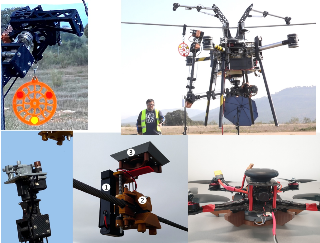
Figure 11: Top) Clip-type bird diverter end effector and installation with MLMP using IMU-based teleoperation method. Bottom-left) Charging station at the end effector. Bottom-center) Fully integrated system of the lightweight charging station (1 - electronics compartment; 2 - split-core current transformer; 3 - V-shaped landing station). Bottom-right) Charging station integrated on HolyBro QAV250 quadrotor, which is used as a proof-of-concept drone to demonstrate the charging of the drone with the developed charging station.
