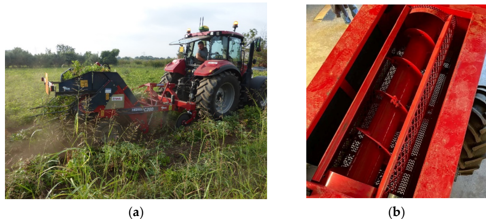
Figure 1. (a) Digging inverter machine adopted. (b) Particulars of the threshing system adopted in separation machine.
