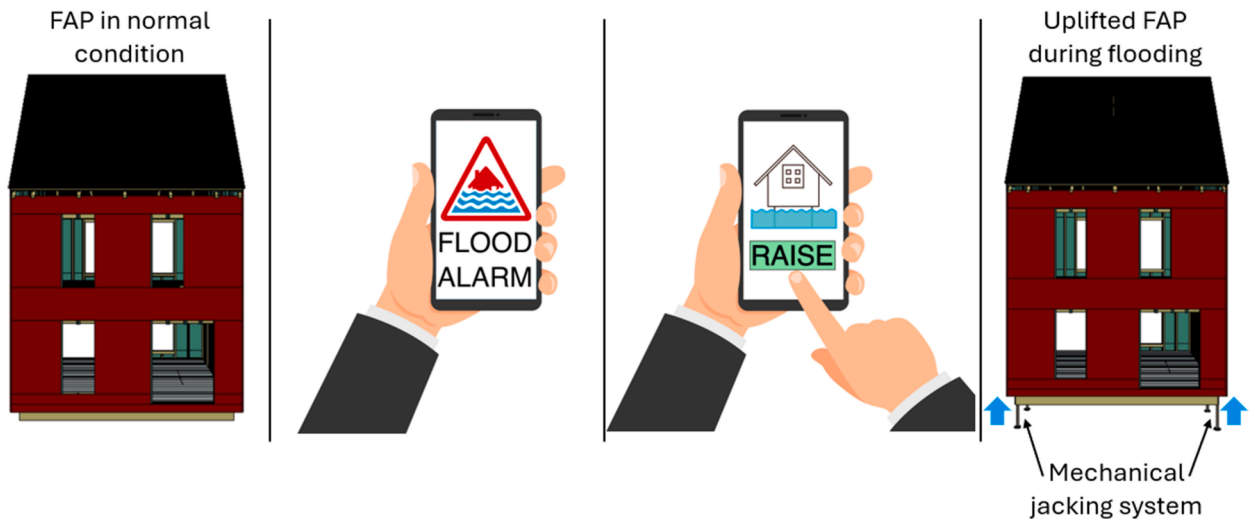
Fig. 4. Remote Flood Adaptive Platform system lifting.
