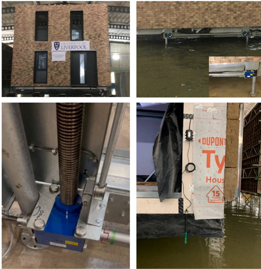
Fig. 6. FAP system tested in full scale at the state-of-art testing facility (HR Wallingford in Oxfordshire, UK).
