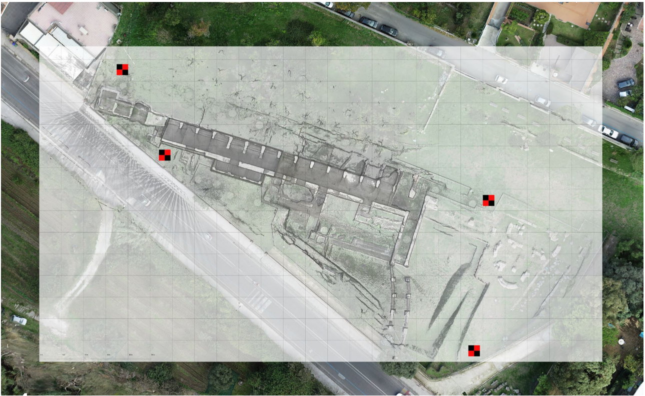
Figure 13. Overlay TLS – RPAS survey of Stadium of Antonino Pio. GCP location.
