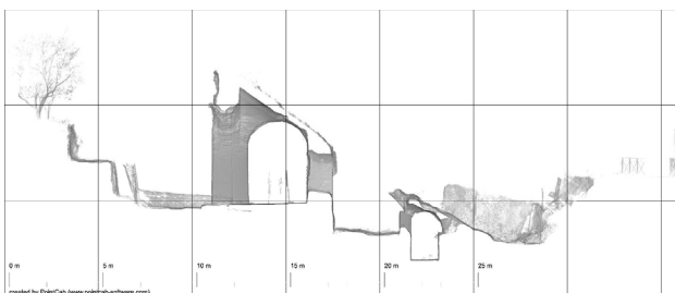
Figure 12. Orthoprojection of section from TLS point cloud of Stadium of Antonino Pio.
