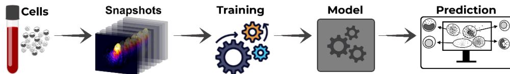
Fig. 5. Working principle of cell class prediction with a CNN model from a fresh blood sample using single cell scattering snapshots. The classifier model is altered for closed- and open-set application to predict known and unknown cell classes at the same time.
