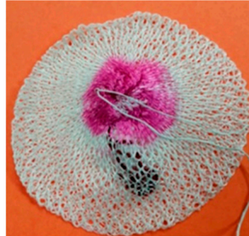
Figure 3. Thorium-containing incandescent lamp mantle.
