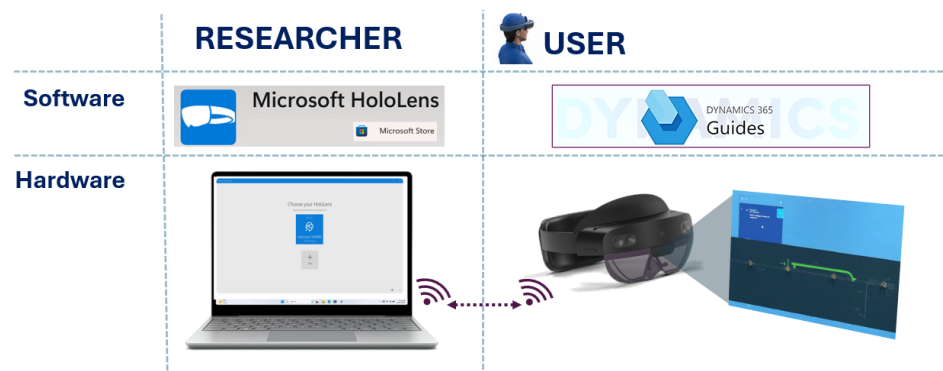
Figure 2. Schema of adopted software and hardware architecture for MR-based technological demonstrator, including equipment for researchers to conduct real-time observation during experiments.
