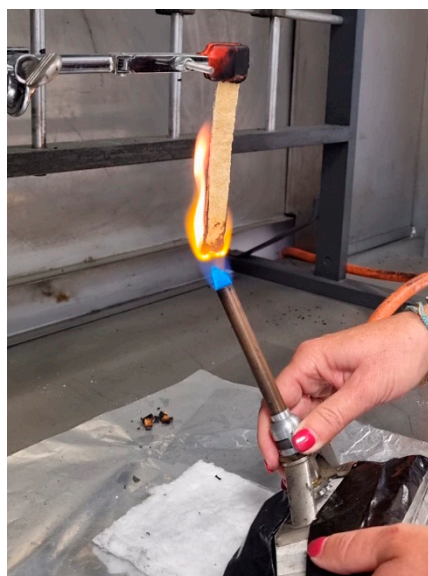
Figure 11. Vertical flammability test setup according to ASTM D3801.
