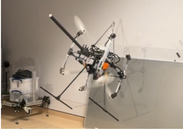
Fig. 4: The octarotor used in experiments during the 30-degree roll maneuver, where the QP-based allocation causes chattering and unrealizable speeds.
