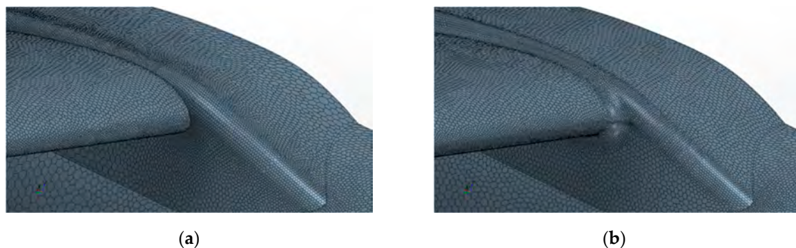
Figure 16. Wing–fuselage fairing geometries without (a) and with (b) fillet.
