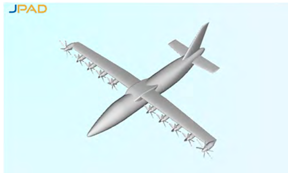
Figure 1. A sketch of aircraft geometry, commuter aircraft 19 pax, obtained by means of JPAD.
