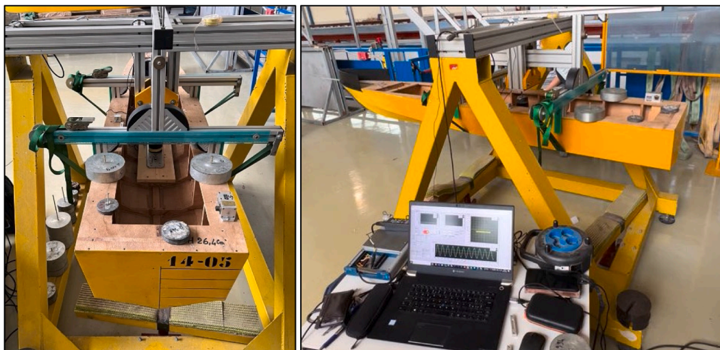
Fig. 2. Determining the CG position and radii of gyration for model C5.
