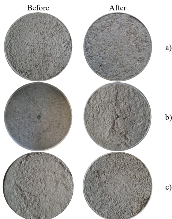
Fig. 5. Photo comparison before and after the evaporation test on the a) dry, b) optimum and c) wet compacted specimens.
