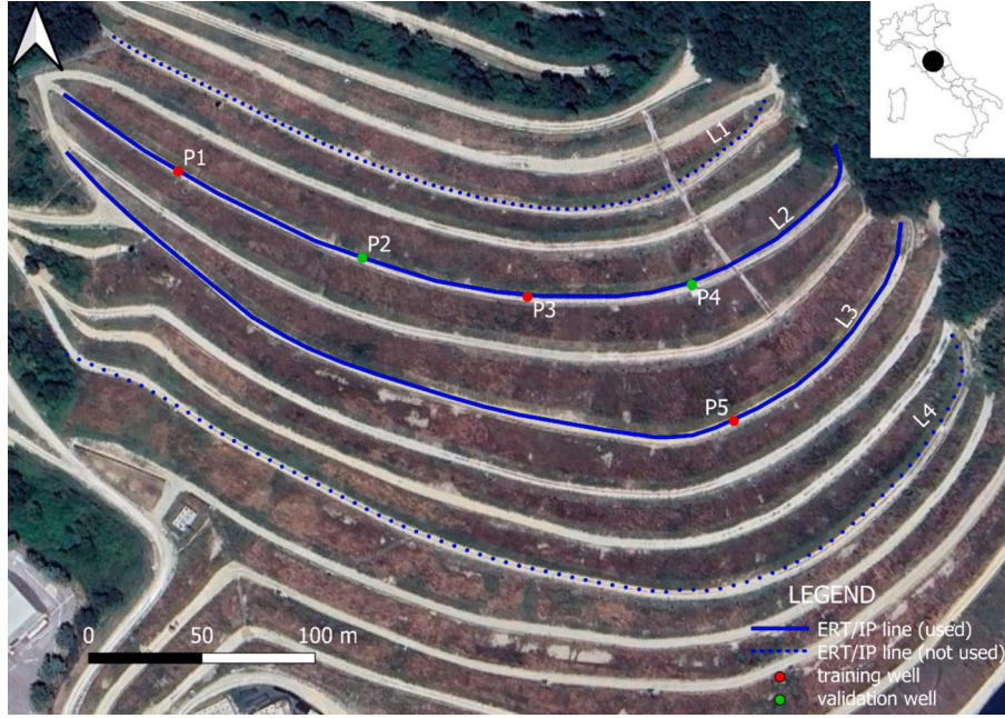
Fig. 2. Aerial view of the landfill site with location of the ERT/IP lines (blue lines). The lines L2 and L3 employed in this work are marked with blue solid lines. The location of wells used for training (piezometers P1, P3 and P5) is marked with red circles, while validation wells (P2 and P4) are marked with green circles. (For interpretation of the references to colour in this figure legend, the reader is referred to the web version of this article.)
