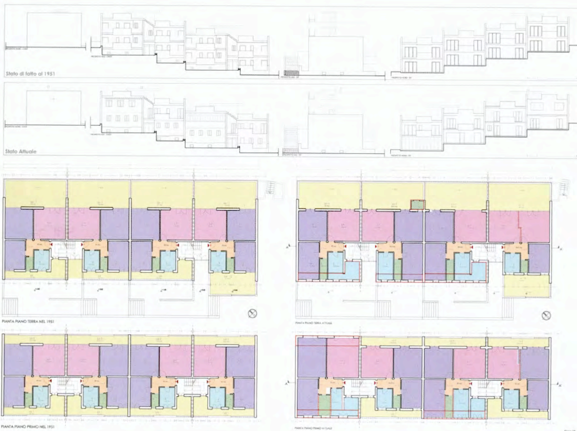
Palazzina 10: existing condition/new condition. Loggias have become verandas.
