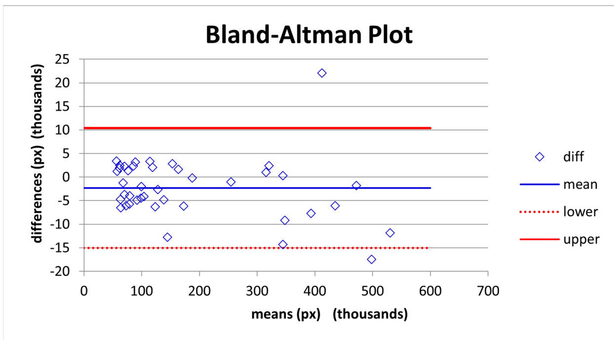
Figure 3. The B&A plot can be evaluated as in good agreement according to the scatter dispersion. The scattering of points is reduced, and points lie relatively close to the line representing mean bias. It is essential to consider the big numerical difference existing among data; this difference in the two outlier cases might (outside the limits of agreement) be due to human error during the Fiji analysis [3].
