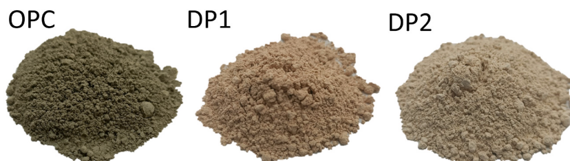
Fig. 1. Image of cement powder and desert sand powders.
