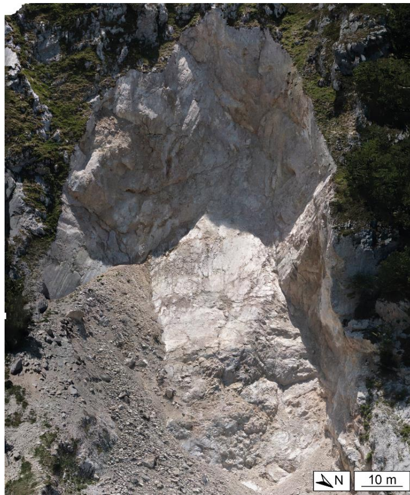
Figure 2. Detail of the Foce rockslide scar from the UAV-derived frontal orthophoto.
