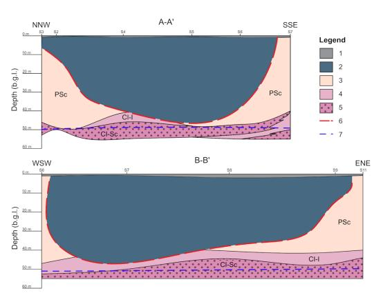
**Figure 4.** NW–SE and SW–NE litho-stratigraphic cross-sections. Traces are taken from Figure 3. Legend: (1) made ground; (2) landfill material; (3) upper pyroclastic deposits (PSc); (4) Campanian Ignimbrite, incoherent facies (CI-I); (5) Campanian Ignimbrite, scoriaceous facies (CI-Sc); (6) bottom of the landfill body reconstructed from geoelectric tomographic profiles; (7) piezometric level (October 2022).
