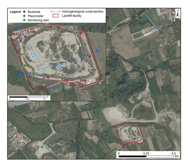
**Figure 3.** Groundwater monitoring network, location of the geognostic surveys (borehole/piezometer logs) and the litho-stratigraphic cross-sections reported in Figure 4. The red polygon delineates the perimeter of the Settecainati-Cava Bianco landfill. Basemap: 2012 aerial photo from http://www.pcn. minambiente.it/mattm/ (accessed on 8 September 2023).
