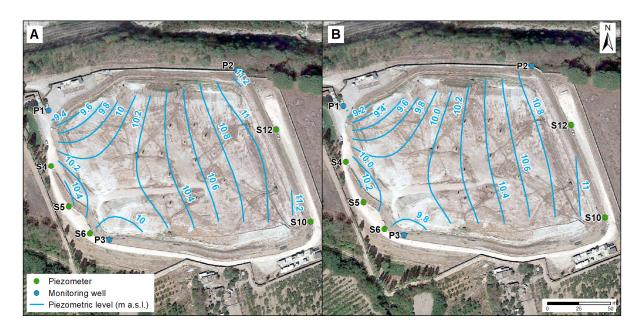
**Figure 5.** Piezometric level of the shallow, unconfined aquifer in June (**A**) and October (**B**) 2022. Basemap: Orthophoto of the landfill area in 2021, provided by S.A.P.NA. S.p.A.
