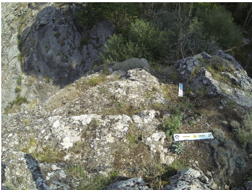
Fig. 3 - Scale bars to support photogrammetric surveys.
