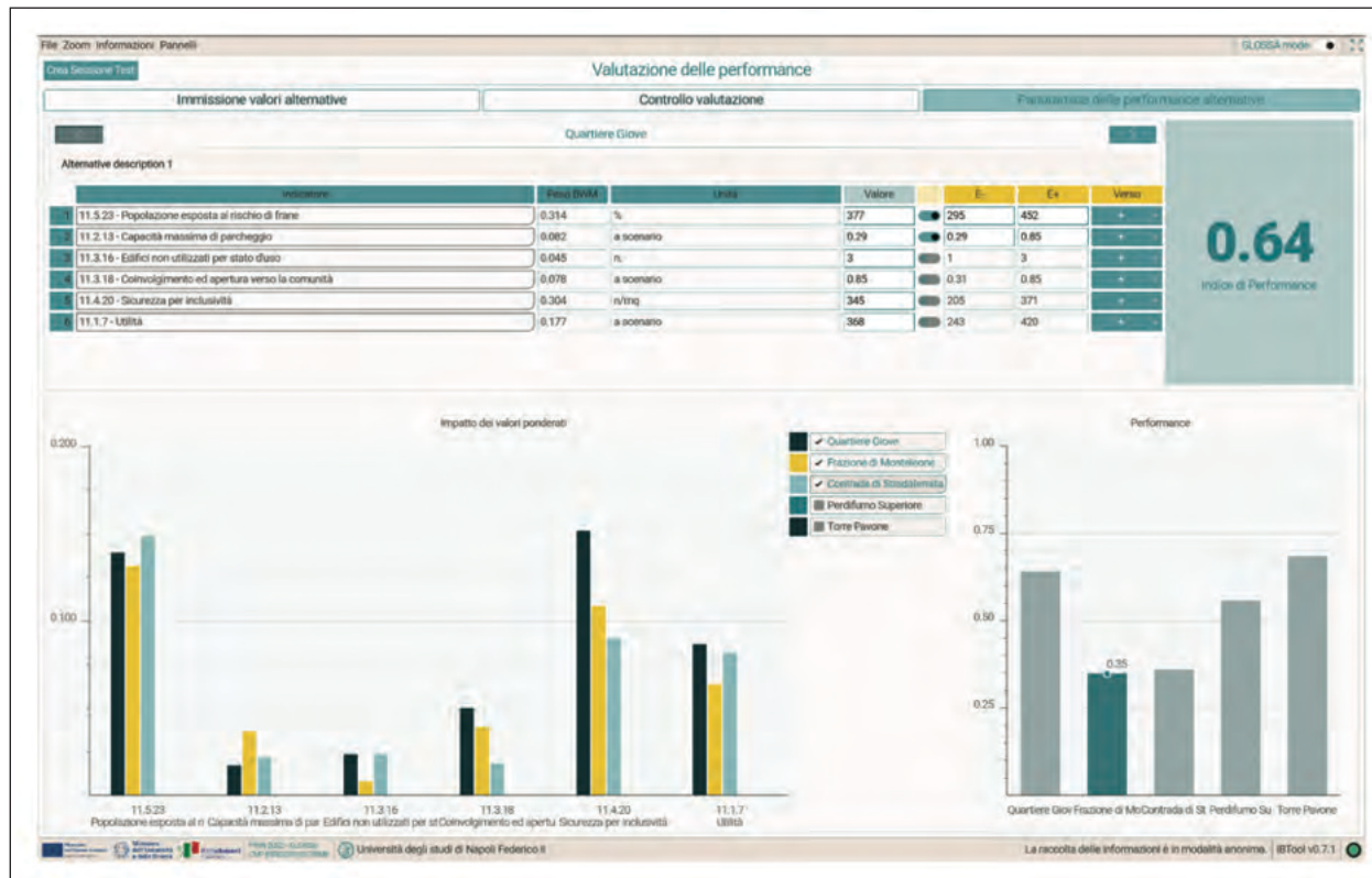
Figure 9. IBTool panel for sustainability performance checking through bar charts (software screenshot).
