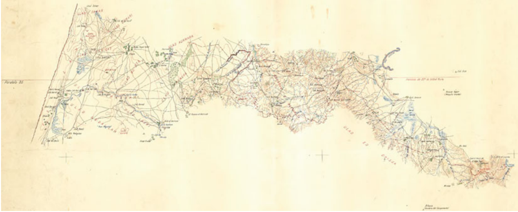
Fig. 9.3 Topographic survey of the border area from the sea to Lucus region. Morocco Boundary Commission. May 1913. Scale 1:50,000. Four color handwritten map on Canson paper. Relief using contour lines. One sheet of
