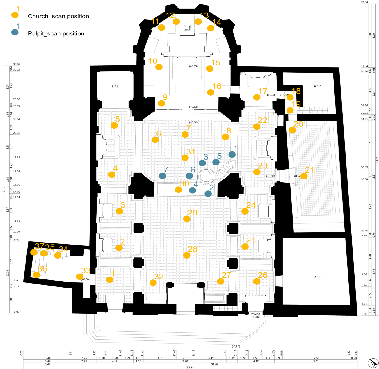
Fig. 2 - Reality-based data acquisition. Schematic drawing of scans positions.
