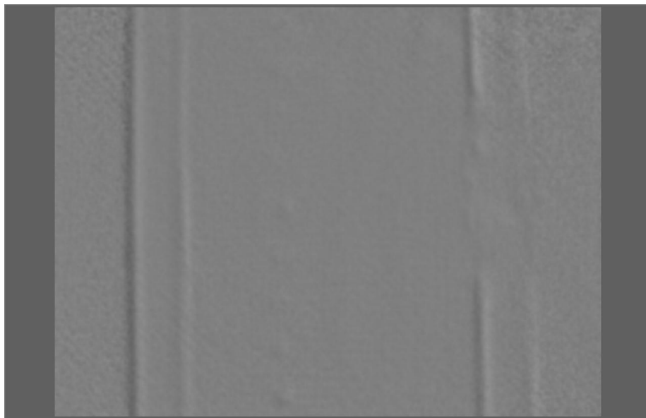
Fig. 7. In plane view of LS map carried out on a whole panel bay consisting in one intact (left) and one debonded (right) stringer.
