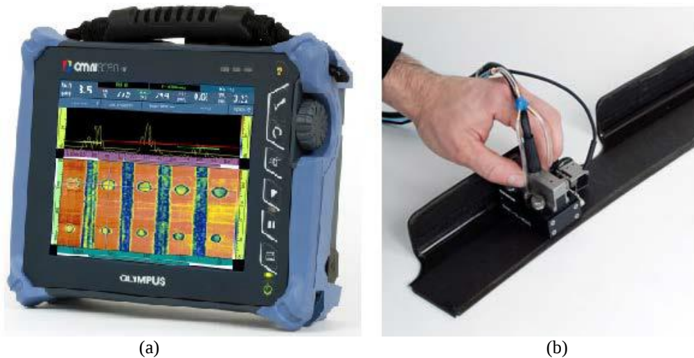
Fig. 2. Olympus OmniScan SX flaw detector (a) equipped with a 16:64PR phased array unit (b) able to perform pulse-echo, pitch-catch or TOFD inspection on composite structures.
