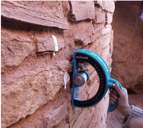
Figure 6. Pendulum rebound hammer test.
