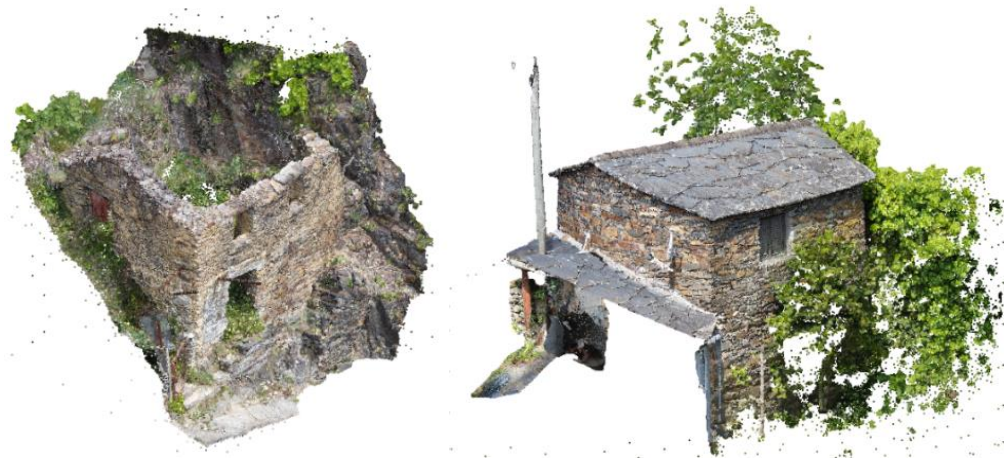
Figure 4. Unified point clouds of the first and second case study, respectively
