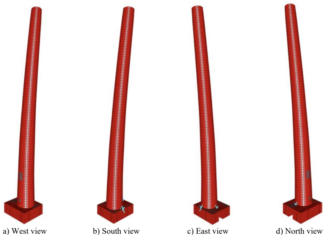
Figure 9. Displacements due to wind action (characteristic values).
