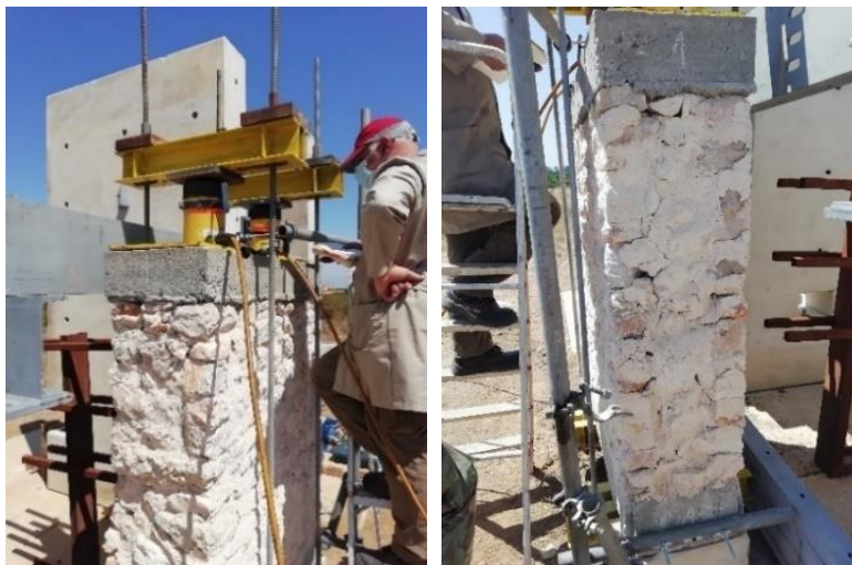
Figure 5. Applying loading system and deflectometer support assembling [1]
