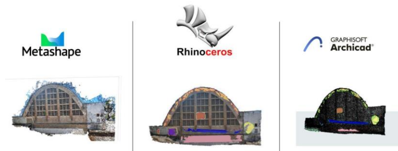
Figure 22. Process of Photoscan to HBIM.
