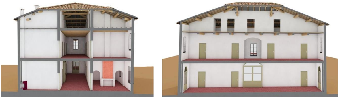
Figure 3. 3D model representing the current state of the villa: cross-section (left) and longitudinal section (right) (© 2020, Habitat Plus).
