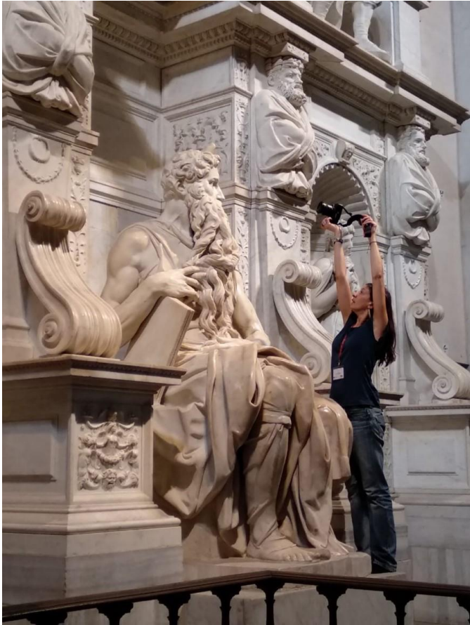
Figure 2. Photogrammetric survey of the statue of the Moses on top of its basis.
