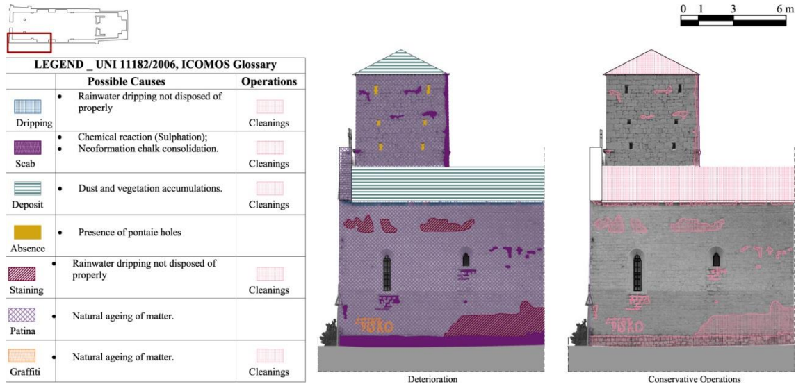
Figure 7. Degradation survey and conservation interventions.
