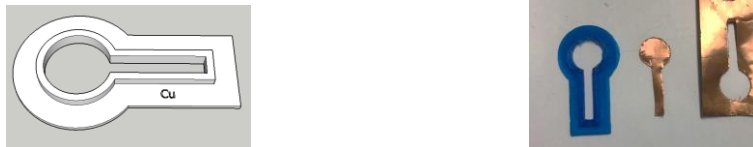
Figure 10: Left: designed 3D-model of the cropping mask. Right: plate #2 cropped from the copper sheet.
