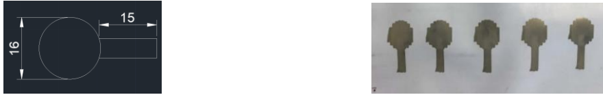
Figure 9: Left: dimensioned CAD drawing of Plate #1. Right: Plate #1 deposited with AJP on the polyurethane substrate.
