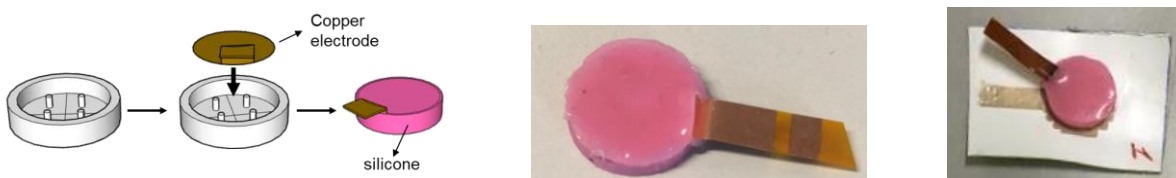
Figure 11: Left: casting mold model and copper electrode placement. Middle: copper electrode (Plate #2) encapsulated in the silicon substrate. Right: realized capacitive force sensor.
