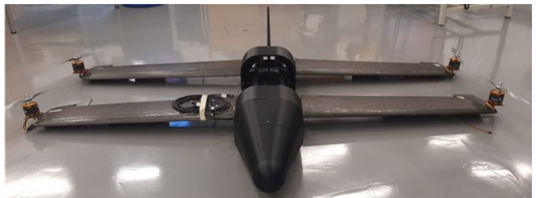
Figure 1. LIBIS—electrically powered UAV designed for versatile aerial operations with a maximum takeoff weight of 25 kg and a wingspan of 2 m.
