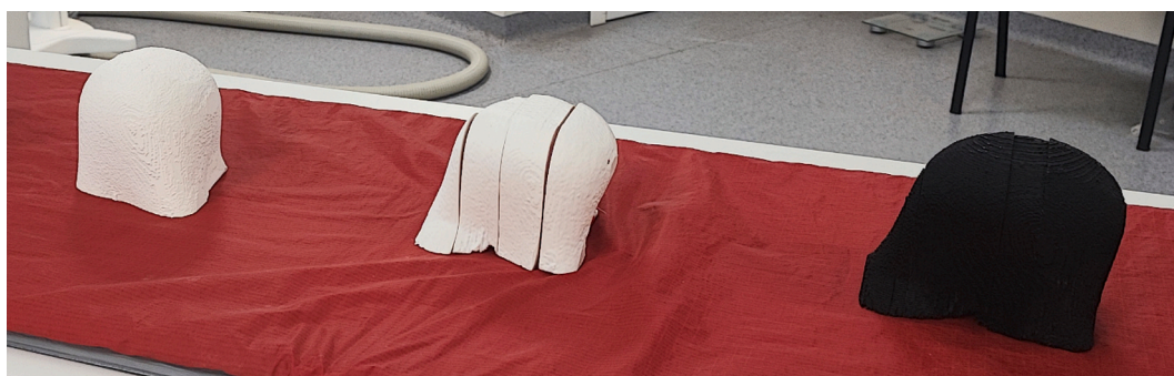
Fig. 3. Printed breast phantoms: (left) Physical breast phantom PB2 from ABS-ASA, (middle) Physical breast phantom PB3 from HIPS-ASA and (right) Physical breast phantom PB1 from PLA.
