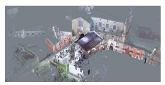
The survey project led to the acquisition of a total number of 36 scans, with 1/8 resolution and 4x quality as settings.
