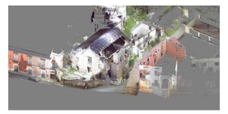
Figures 5-6. Point cloud from laser scanner survey.
