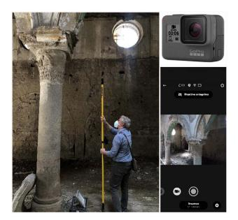
Figure 10. Terrestrial photogrammetric survey activities.
