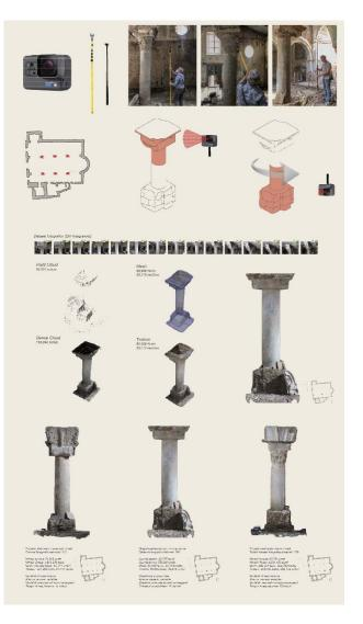
Figure 11. Photogrammetric survey of the columns.
