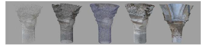
Figure 12. Processing of the photographic datasets of the internal capital.
