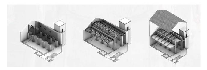
Figure 15. Model of the church pre-earthquake. Graphic elaboration by Mariarosa Sarracco.
