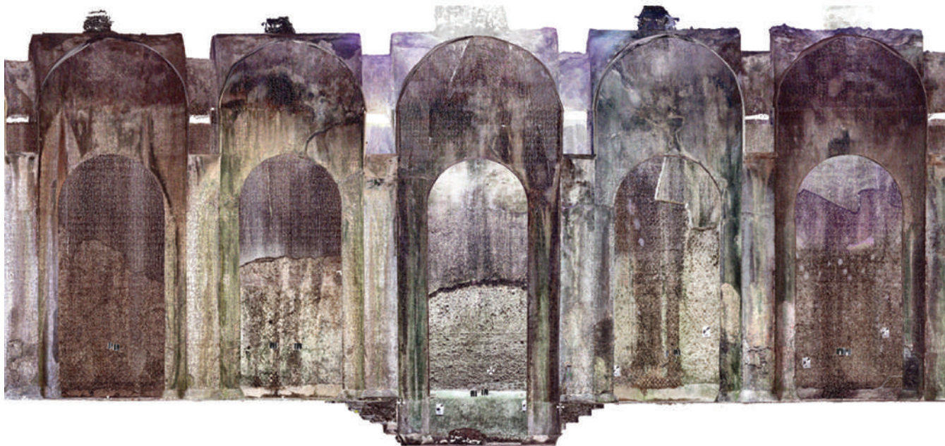
Figure 7. Partial cross-section showing the central part of the Piscina Mirabilis, as a result of TLS data processing in FARO Scene software.
