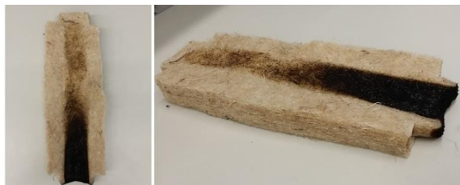
Figure 8 : Flammability test of Untreated Hemp fibers
