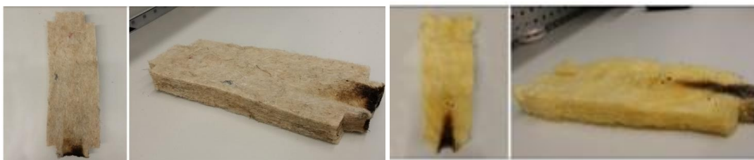
Figure 9 : Flammability test of Treated Hemp fibers (left) – Glass fibers (right)
