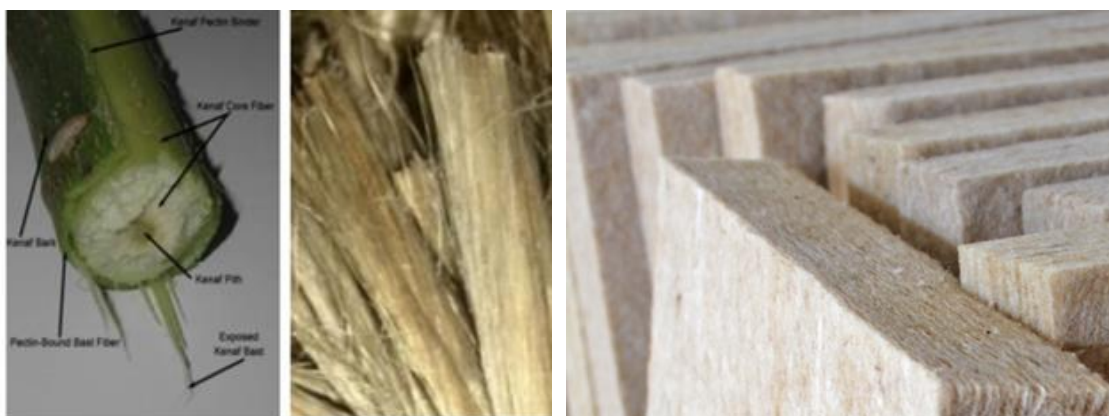
Figure 4 : Hemp straw, fibers and panel
