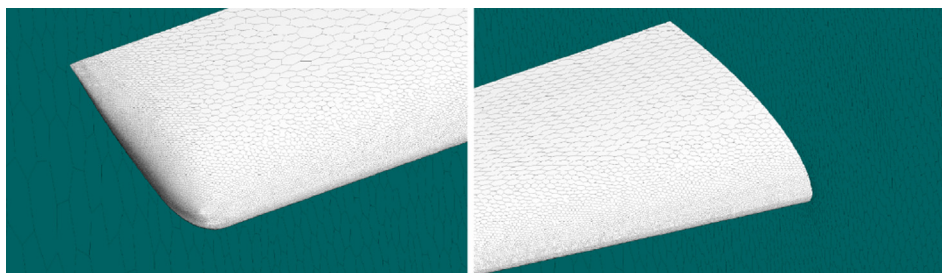
Fig. 8 Close up views of refined surface mesh: (Left) canard tip and (Right) wing leading edge at intersection with the symmetry plane. Rounded tips and surface grid refinement automatically generated with the JPADCAD geometry processing tool 29 coupled to STAR-CCM + 30 automation features.
