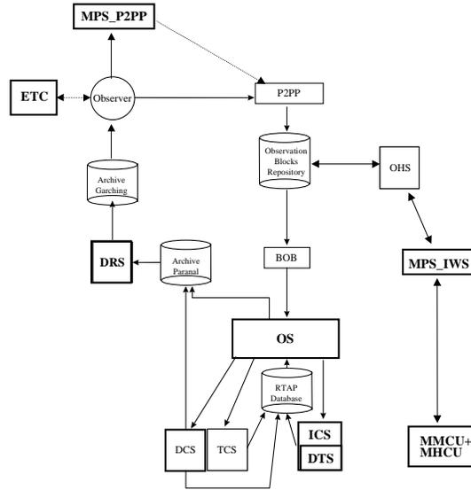
Fig. 1. Layout of VIMOS software : bold objects are VIMOS s/w subsystems. Continuous lines represent direct connections, dashed lines indirect connections between software subsystems
