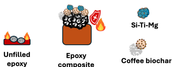
Figure 2: Flame retardant action of additives in the condensed phase during the combustion
