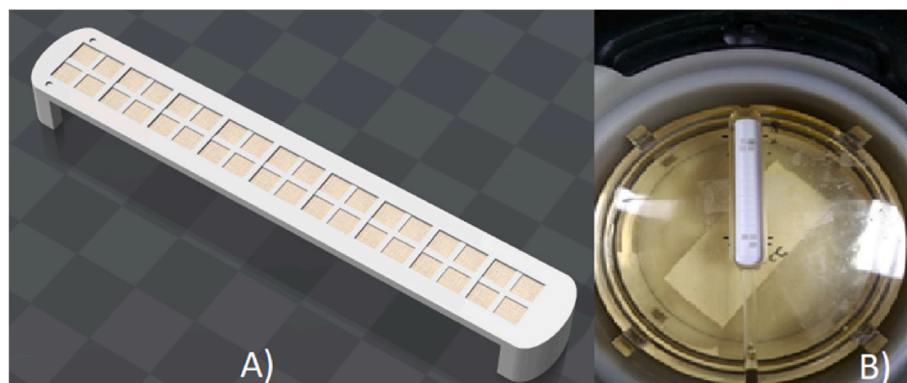
Fig. 4. ASA support A) for TLDs housing; B) inserted in the PMMA phantom.
